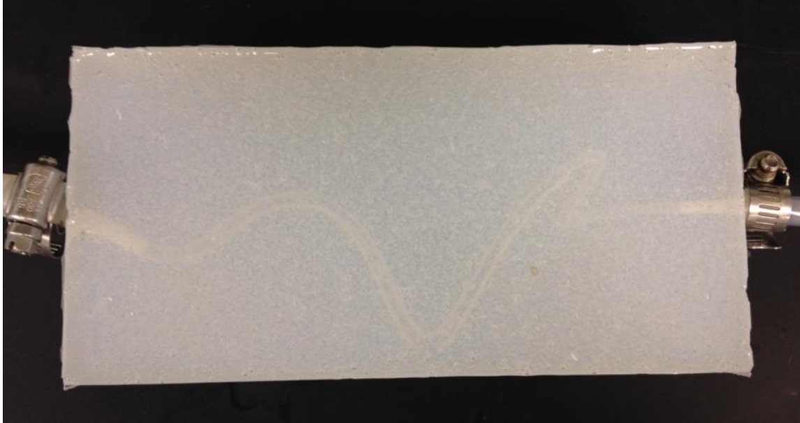
Figure 20. First prototype of silicone vessel model
